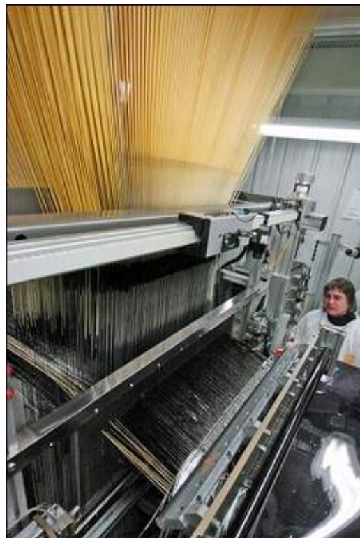
Albany Engineered composites technician Susan West works a 3-D weaving machine at the Rochester facility Monday. (John Huff/Staff photographer)
